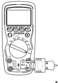
**Note:** The temperature probe is fitted with a type K mini connector. A mini connector to banana connector adaptor is supplied for connection to the input banana jacks.
